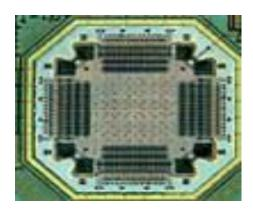
Micro-electromechanical systems (MEMS) incorporate miniature electro-mechanical components fabricated with processing techniques and equipment originally developed in the semiconductor industry.
